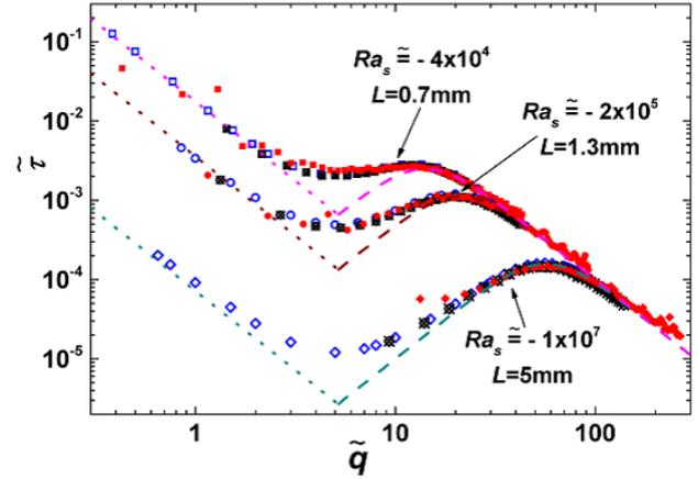
**Fig. 5.** Decay times of non-equilibrium concentration fluctuations in a binary mixture of 1,2,3,4-tetrahydronaphtalene and *n*-dodecane subjected to a stabilizing temperature gradient. Different symbols are for different thicknesses of the sample cell, thus resulting in different solutal Rayleigh numbers. Figure reproducing data already published in [77].
