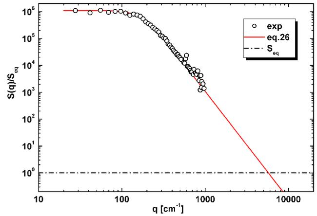
**Fig. 1.** Intensity  $S(q)$  of the non-equilibrium concentration fluctuations during free diffusion in an aqueous solution of urea, relative to the intensity  $S_{eq}$  of the local equilibrium concentration fluctuations, from a reanalysis of data earlier reported in [63].
