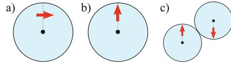
**Fig. 1.** Sketches of spherical particles with a fixed net magnetic moment (red arrow) that is shifted a) laterally or b) radially away from the particle center (black dot). c) Two particles with radial shift form a dumbbell with a non-collinear, antiparallel magnetic order.
