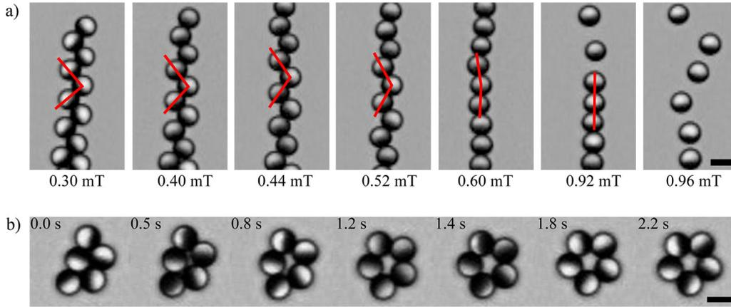
**Fig. 6.** Transformation of particle clusters while exposed to an oscillating out-of-plane field. a) Reversible expansion of a staggered chain under increasing field amplitudes  $B_0^{\text{ex}}$  as noted below the images ( $\omega = 10\pi$  Hz). b) Time sequence of the abrupt transition of a compact cluster into a ring ( $B_0^{\text{ex}} = 1.6$  mT,  $\omega = 38\pi$  Hz). The time is noted in the images (scale bar:  $5 \mu\text{m}$ ).
