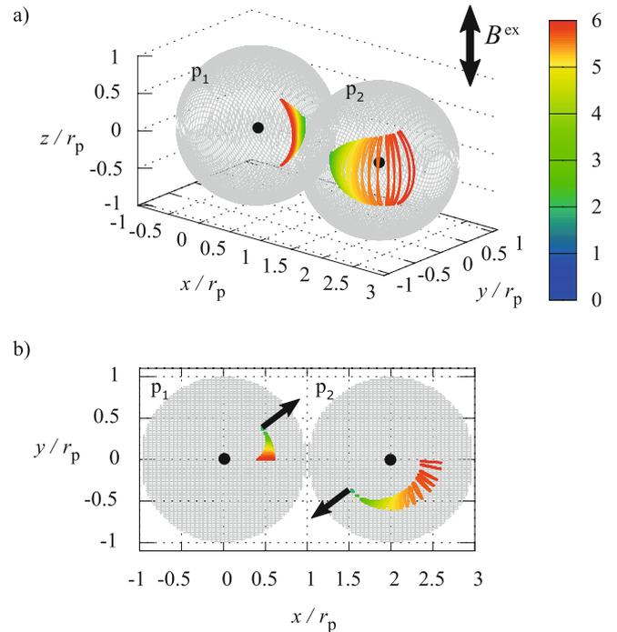
**Fig. 3.** Steady-state oscillations of two interacting sd-particles  $p_1$  and  $p_1$  ( $\xi = 0.6$ ) in oscillating fields  $B^{\text{ex}}$  in a) a three-dimensional view and b) the top view. The trajectories display the trace of the dipole position. The color coding corresponds to the field amplitude  $B_0^{\text{ex}}$  measured in  $\frac{\mu_0 m}{32\pi r_p^3}$ .
