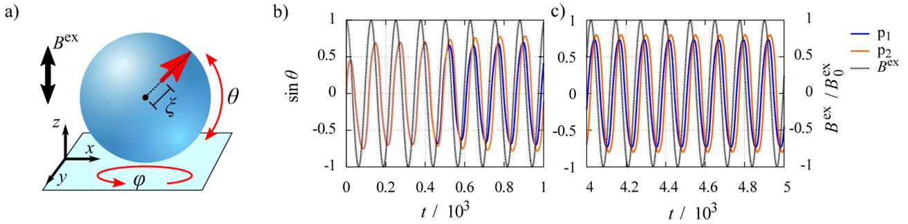
**Fig. 2.** a) The orientation of sd-particles with dipole shift  $\xi$  in the  $xy$ -assembly plane is given by the radial angle  $\theta$  and the azimuthal angle  $\varphi$ . Oscillating fields  $B^{\text{ex}}$  are applied vertically ( $z$ -axis). b) Transient radial oscillation  $\theta(t)$  (left axis) of two sd-particles  $p_1$  and  $p_2$  ( $\xi = 0.6$ ) in contact after a field  $B^{\text{ex}}$  (right axis) is switched on and c) steady-state oscillation after some time.
