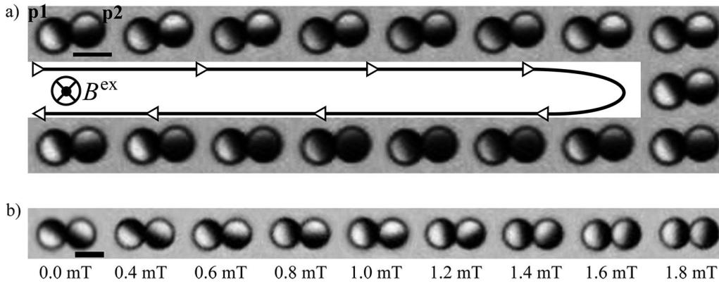
**Fig. 5.** Microscopy images of two capped particles in contact while exposed to an oscillating out-of-plane field  $B^{ex}$  ( $\omega_B = 38\pi$  Hz). a) Time sequence during one field cycle ( $B_0^{ex} = 0.7$  mT). b) Snapshots of two particles at different field amplitudes  $B_0^{ex}$  given below the images. (Scale bar:  $5 \mu\text{m}$ ).
