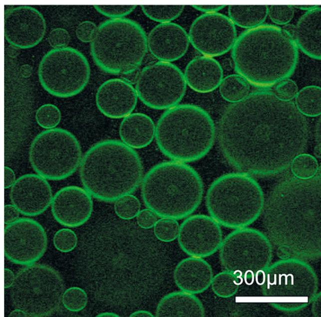
**Fig. 13.** Confocal fluorescence micrograph of water-in-toluene emulsion droplets stabilized by the cooperative interfacial segregation of acid-treated SWCNTs and PS-NH<sub>2</sub>. The SWCNTs are fluorescently labeled. ( $C_{\text{PS-NH}_2} = 0.1$  mg/ml,  $C_{\text{SWCNT}} = 0.08$  mg/ml, PS-NH<sub>2</sub>  $M_n = 2,800$ ). Reprinted with permission from *Langmuir* [23] © (2014) American Chemical Society.
