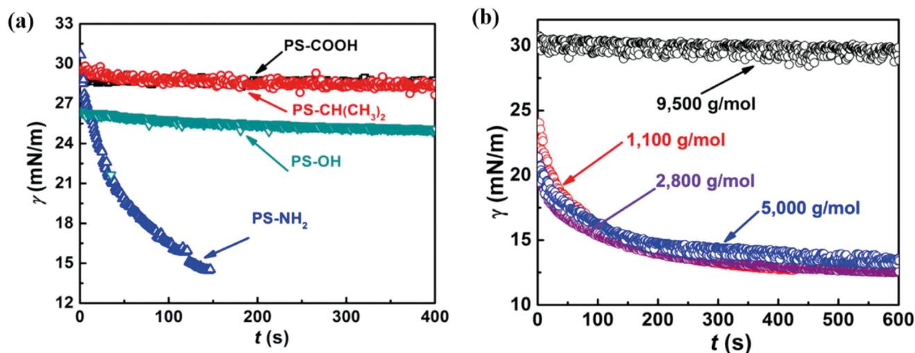
**Fig. 14.** (a) Impact of PS end-group chemistry on the time evolution of interfacial tension  $\gamma$  (PS  $M_n \sim 2,000$  g/mol,  $C_{PS} = 0.5$  mg/ml,  $C_{SWCNT} = 0.08$  mg/ml,  $pH \sim 3.5$ , 6 h SWCNT acid treatment). (b) Impact of PS-NH<sub>2</sub> molecular weight on the time evolution of interfacial tension  $\gamma$  (PS-NH<sub>2</sub>  $M_n \sim 2,800$  g/mol,  $C_{PS} = 0.5$  mg/ml,  $C_{SWCNT} = 0.08$  mg/ml,  $pH \sim 3.5$ , 6 h treated SWCNTs).
