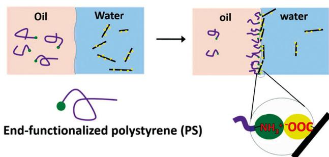
**Fig. 11.** Cooperative interfacial segregation between acid-treated SWCNTs and PS-NH<sub>2</sub>.
