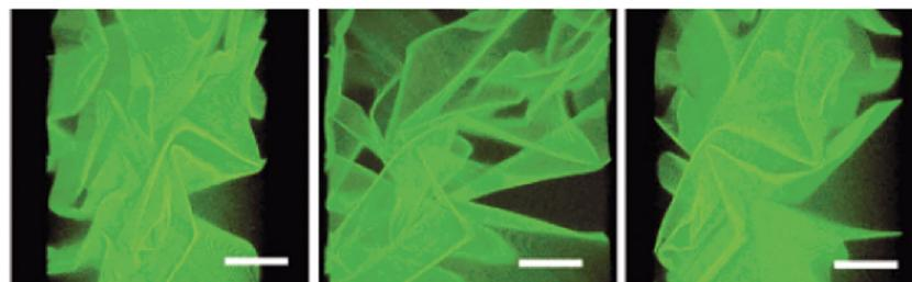
**Fig. 6.** Confocal microscopy image of a nanoparticle sheet prepared by cross-linking the vinyl benzene ligands. The scale bar is 50  $\mu\text{m}$ . Reprinted with permission from *J. Am. Chem. Soc.* [11] © (2003) American Chemical Society.
