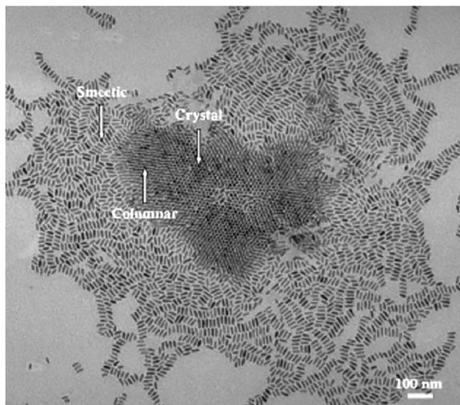
**Fig. 8.** TEM image of a TOPO-covered CdSe-nanorod-stabilized water droplet after drying on a carbon-coated copper grid. Reprinted with permission from *Small* [12] © (2007) John Wiley and Sons.
