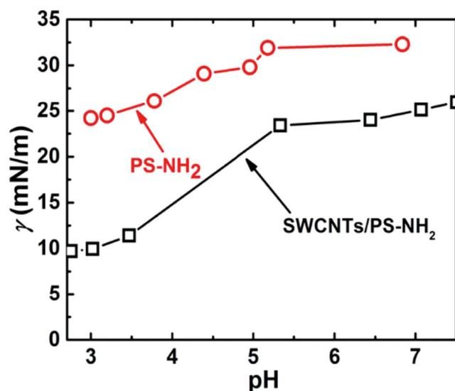
**Fig. 15.** Steady-state  $\gamma$  as a function of SWCNT solution  $pH$  (red: without SWCNTs in aqueous phase; black: with SWCNT in aqueous phase,  $C_{\text{SWCNT}} = 0.5 \text{ mg/ml}$ , initial  $pH \sim 2.7$ ).
