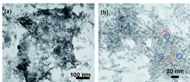
**Fig. 10.** TEM images of a cross-linked sheet made by co-assembly of ferritin and CdSe nanorods at a chloroform-water interface (a) low magnification image, and (b) high magnification image showing individual CdSe nanorods (red ovals) and ferritin particles (blue circles). Reprinted with permission from *Soft Matter* [17] © (2009) Royal Society of Chemistry.
