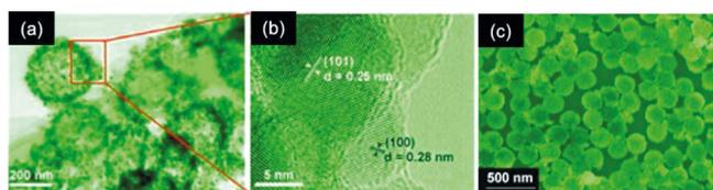
**Fig. 4.** Typical (a) TEM and (b) HRTEM images of the ZnO hollow spheres. (c) SEM image of the ZnO hollow sphere nanofilm deposited on a  $\text{SiO}_2/\text{Si}$  substrate. Reprinted with permission from *Small* [9] © (2011) Wiley-VCH.
