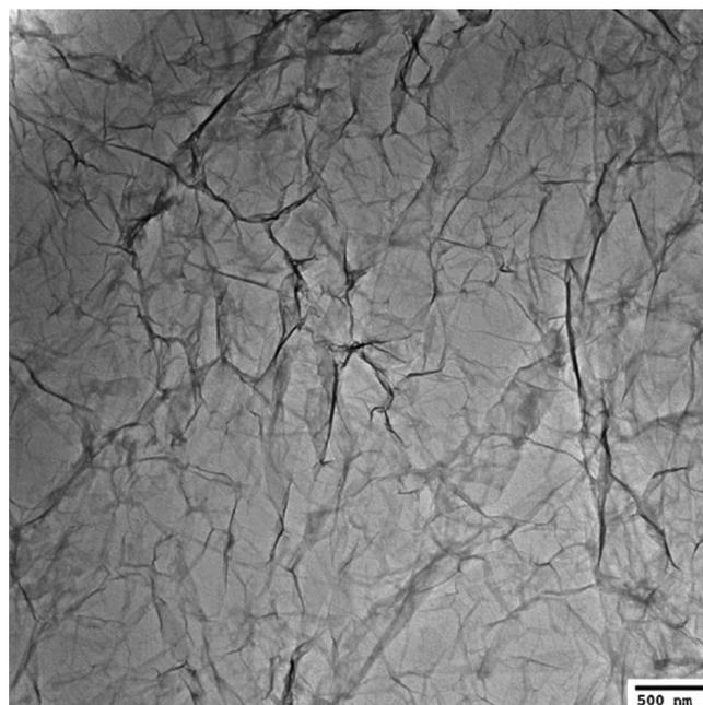
**Fig. 19.** TEM image of the assembled graphene film at the toluene/water interface. Reprinted with permission from Langmuir [24] © (2013) American Chemical Society.
