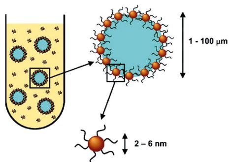
**Fig. 1.** Schematic of self-assembly of nanoparticles at a fluid-fluid interface. Reprinted with permission from *Langmuir* [2] © (2005) American Chemical Society.
