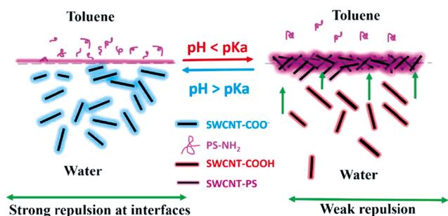
**Fig. 16.** Physical depiction of  $pH$ -induced, SWCNT segregation transition at the toluene/water interfaces (2003) American Chemical Society.
