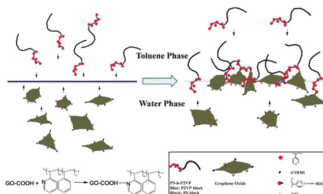
**Fig. 17.** Assembly of graphene oxide and block copolymer at the toluene/water interface. Reprinted with permission from *Langmuir* [24] © (2013) American Chemical Society.
