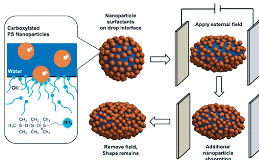
**Fig. 20.** Schematic representation of the deformation of a spherical drop, clad with nanoparticle surfactants, by an electric field, into an ellipsoid whose shape is maintained after the removal of the field by the interfacial jamming of the nanoparticle surfactants. Reprinted with permission from Science [25] © (2013) The American Association for the Advancement of Science.
