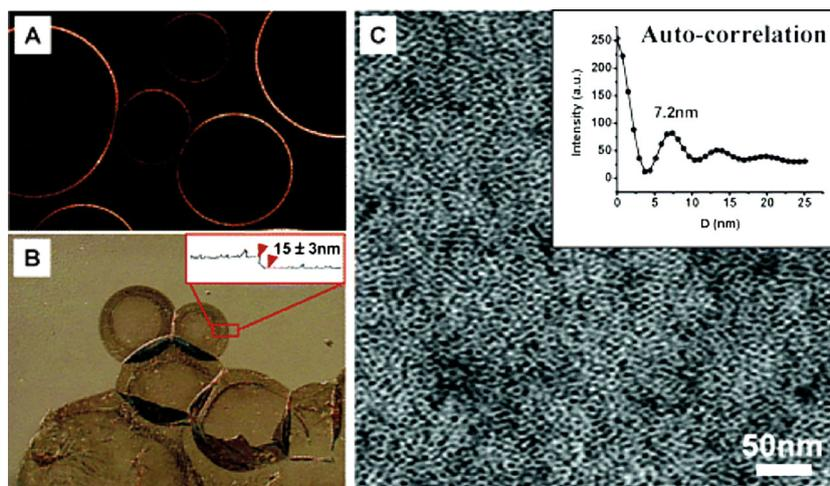
**Fig. 5.** (A) Fluorescence confocal microscopy image of CdSe nanoparticles covered water droplets dispersed in toluene. (B) Differential interference contrast optical microscopy image of dried droplets on a silicon substrate. Inset: AFM height section analysis. (C) TEM image of a dried droplet. Inset: Autocorrelation function of the TEM image. Reprinted with permission from *Langmuir* [2] © (2005) American Chemical Society.
