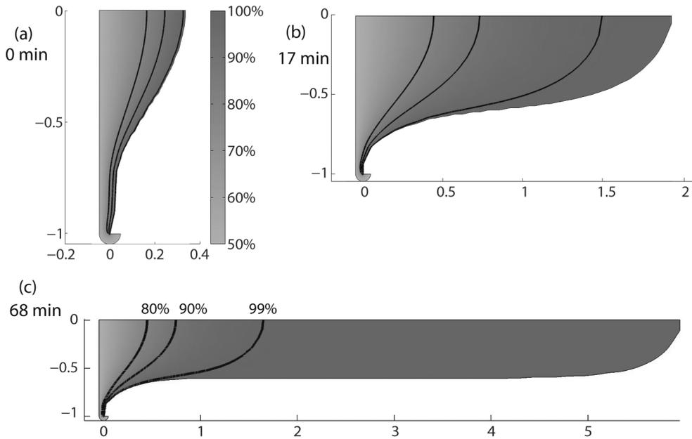
**Fig. 6.** Fields of relative humidity  $n/n_0$  for the observed air/water interfaces as shown in fig. 3 (axes scale is millimeter). The air is saturated with water at the air/water interface and  $n/n_0 = 50\%$  at a distance  $\delta$  from the channel entrance (light gray); as shown in fig. 2. The gray scale is common to all figures. The black lines indicate curves of iso-humidity (80, 90 or 99%).
