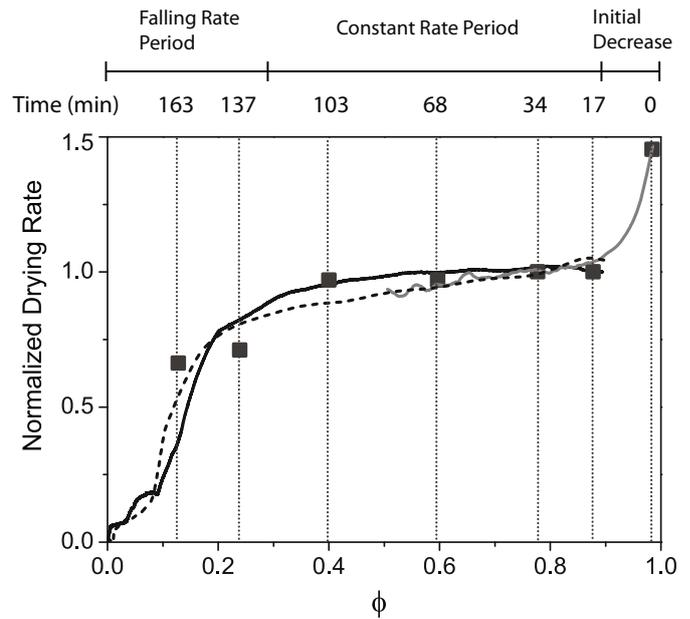
**Fig. 5.** Drying rate, normalized at CRP, as a function of the saturation, from two measurements by TGA (black continuous and dotted curves) and from image analysis (gray curve). Times refer to pictures of fig. 3. The gray squares are the drying rate computed from FEM.
