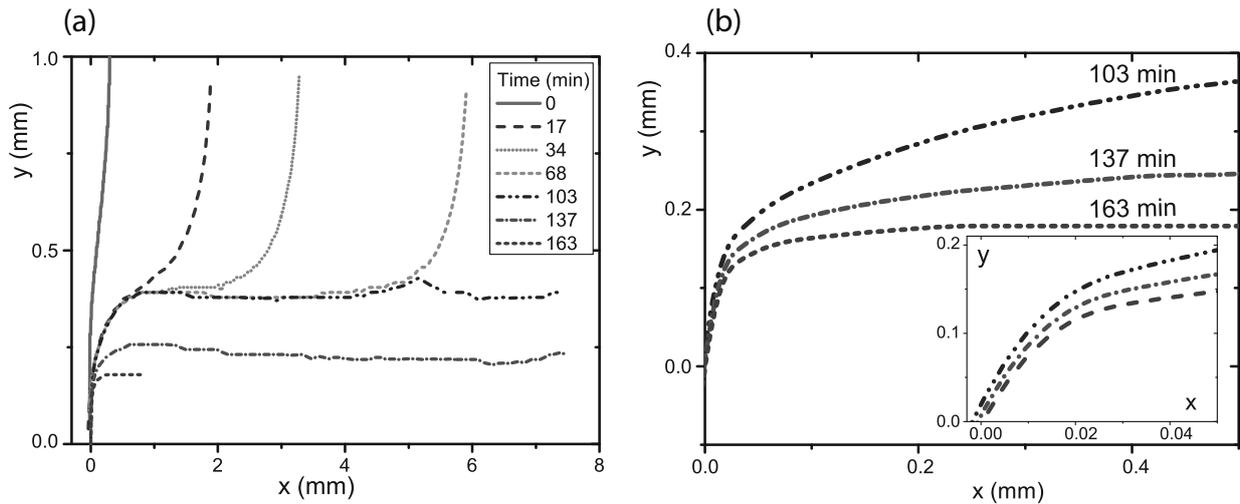
**Fig. 4.** (a) Shape of the air/water interface for images from fig. 3, drying times are indicated in minutes. We present here the upper half of the images of the interface. The channel is open at  $x = 0$  and its axis is  $y = 1$  mm. (b) Interface close to the entrance of the channel at the end of the drying. The inset is a zoom on the first  $50 \mu\text{m}$  of the channel entrance for the same interfaces.
