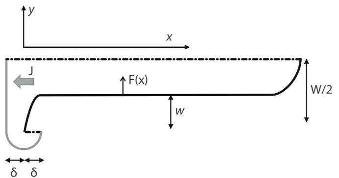
**Fig. 2.** Schematic of the domain used for 2D FEM modeling. The air-water interface is shown as a solid black curve, and the dashed lines indicate no-flux boundary conditions. The humidity is fixed at 50% for the gray curve, which is a distance  $\delta$  away from the channel.  $F$  is the local evaporation from the interface and the drying rate  $J$  is the flux of water vapor through the channel entrance.
