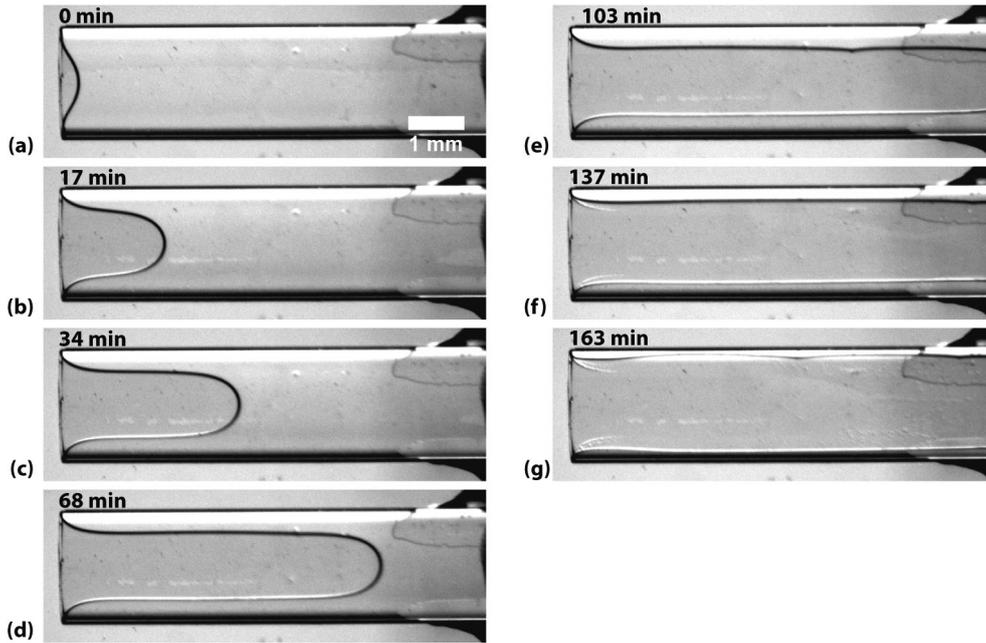
**Fig. 3.** Top views of the channel (open on the left) at different times during drying: (a) initial and after 17 (b), 34 (c), 68 (d), 103 (e), 137 (f) and 163 min (g). The scale bar denotes 1 mm and applies to all panels.
