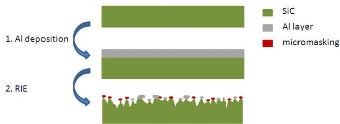
**Fig. 28.** Two-step processing to fabricate nanostructures using Al thin films: (1) Al deposition and (2) reactive ion etching.
